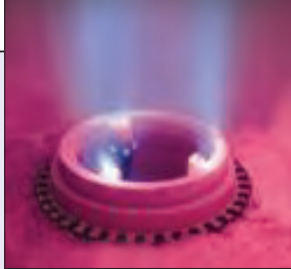
FIGURE 2. GLSF Free-Jet Burner, a next generation ultra-low emissions round-flame burner, offers a design that uses the free-jet method of mixing the fuel gas ejected from the gas tips with the surrounding inert products of combustion to dramatically lower thermal NO x production
