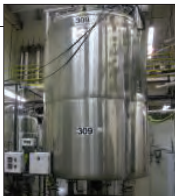
FIGURE 2. Many bio-chemicals are produced in fermenters, like this one at ZeaChem, but some companies are pursuing catalytic methods
